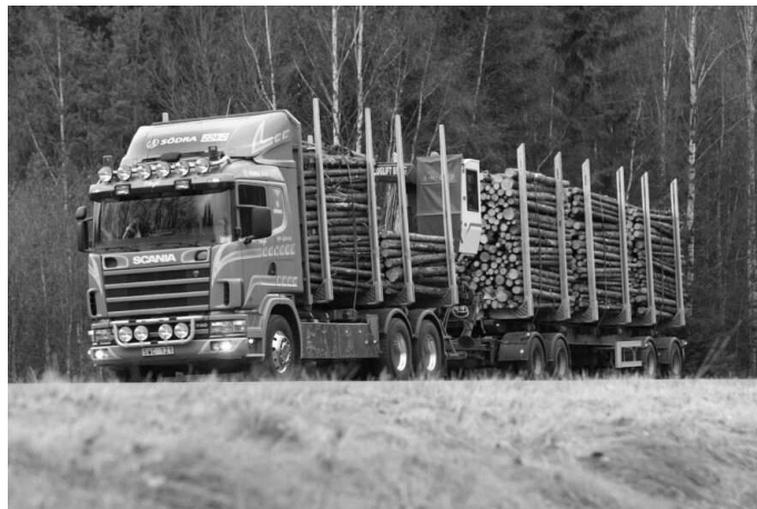
Figure 1: A truck specialized for roundwood haulage. In this case with its own crane loading and unloading
