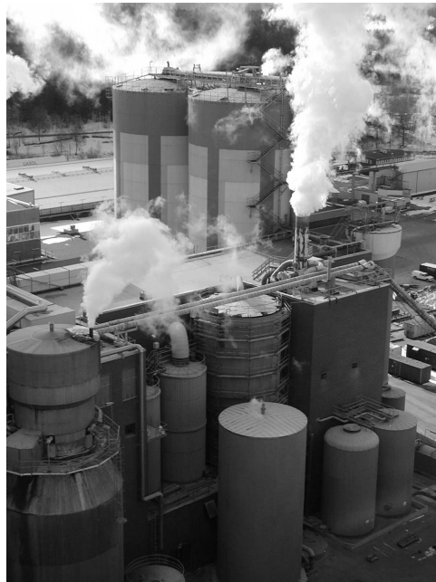
Figure 2 Photo of the bleaching towers used in the four stages at Billerud AB's paper mill in Skärblacka. Photo by Billerud AB.
