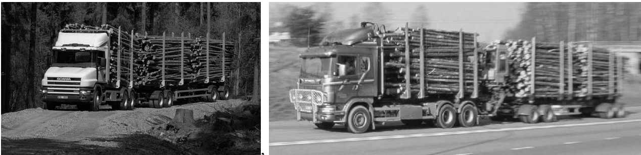
Figure 3: Examples of a standard truck without a crane (left) and with a crane (right).
