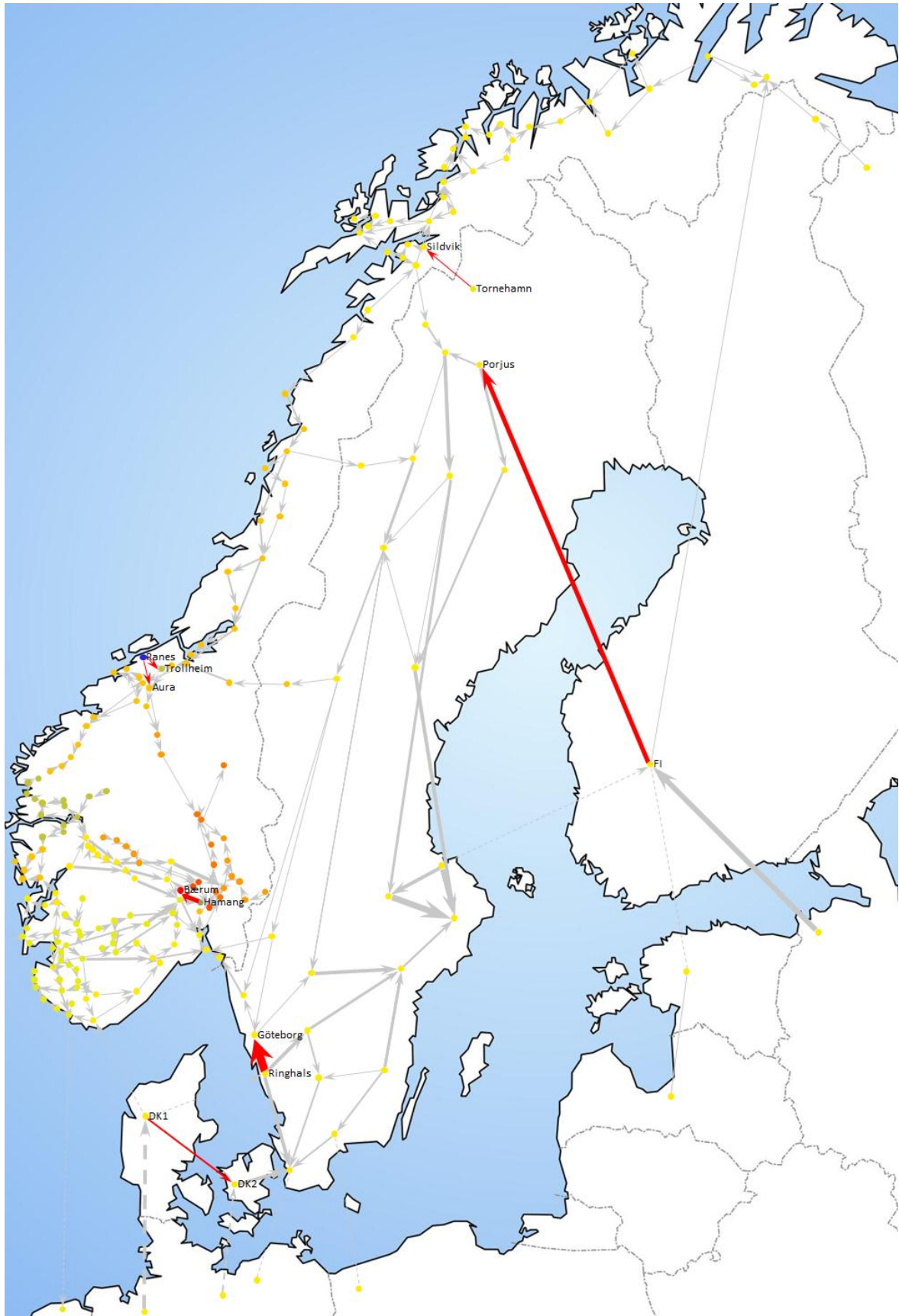
Figure 7-9 Line flows and thermal bottlenecks for optimal nodal price solution, 6/1-2010, hour 10
