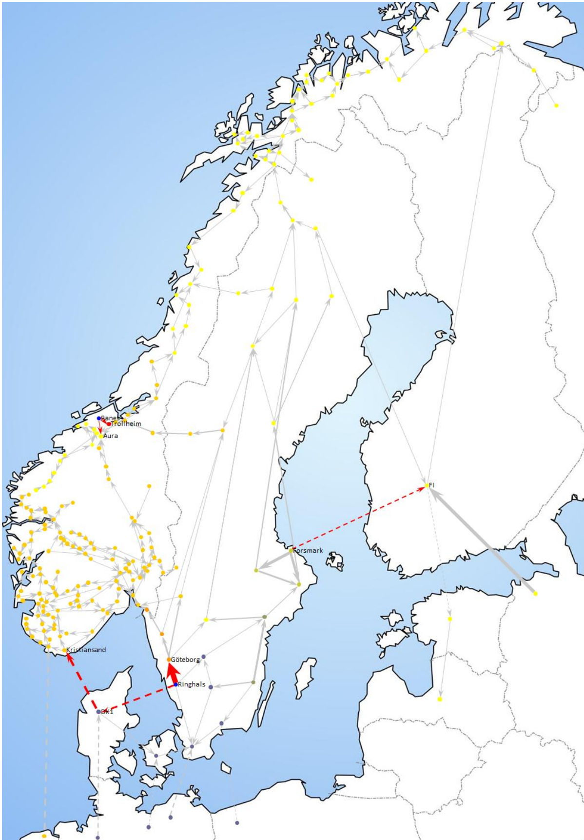
Figure 6-10 Line flows and thermal bottlenecks for optimal nodal price solution, 1/8-2010, hour 6
