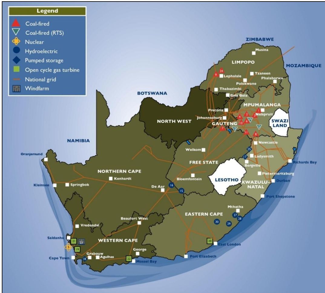
Figure 15: Eskom’s transmission grid and power stations in South Africa (Eskom Website, 2009)
