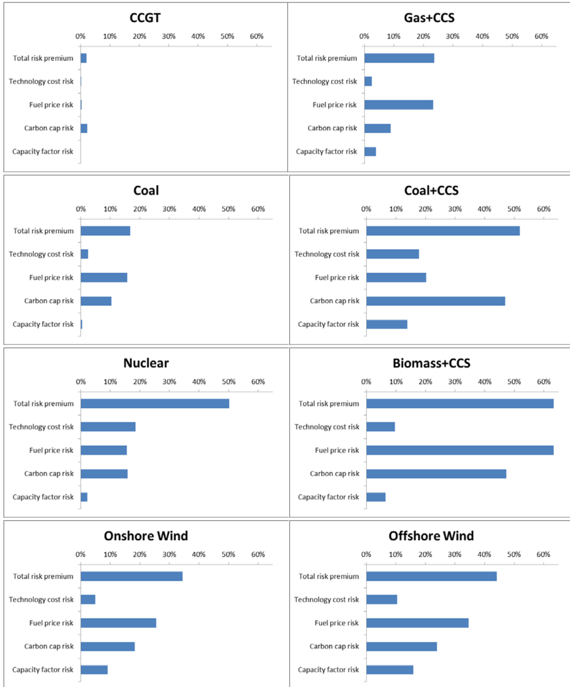
Figure 3. Sources of risk: measured as % increase in revenue required to overcome option value 7
