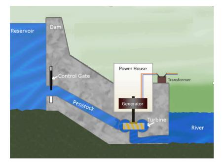
Figure 1: Illustration of hydroelectricity plants
