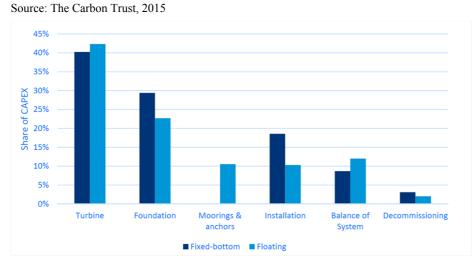
Figure 3-2: Cost breakdown for a typical fixed and floating wind farm
