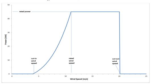
A wind turbine only starts to generate at about 4m/s, and should not generate at speeds above 20-25m/s for safety reasons and to avoid excessive wear and tear of the material. The ideal speed for a wind turbine depends on the turbine's capacity but generally falls between 11m/s and 14m/s.
