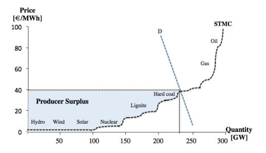
*Figure 3.6:* Infra-marginal rent *Source:* Author's own illustration based on figure from Genoese et al. (2015), Stoft (2002).
