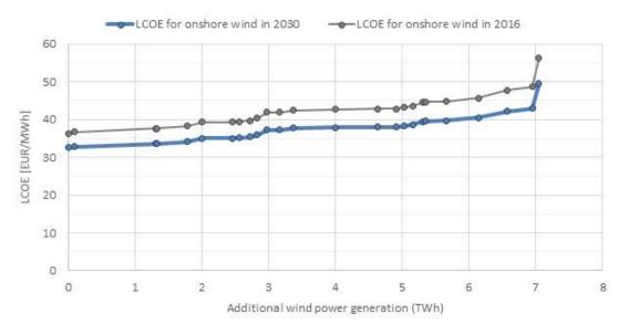
*Figure B.2:* LCOE curves for onshore wind in Norway in 2016 and in 2030 Note: The LCOE curve for 2030 assumes a 15 % decline in the investment costs. Source: Author's own illustration
