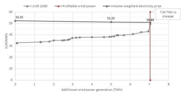
*Figure 5.12:* The wind price and the levelized cost of electricity for onshore wind in Norway in the Moderation Scenario *Source:* Author's own illustration
