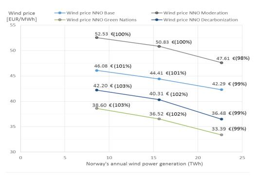
*Figure 5.16:* Wind prices and market value factors (in parenthesis) in Northern Norway under different levels of wind development in the four scenarios *Source:* Author's own illustration
