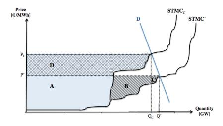
*Figure 3.8:* Change in producer surplus under carbon pricing *Source:* Author's own illustration
