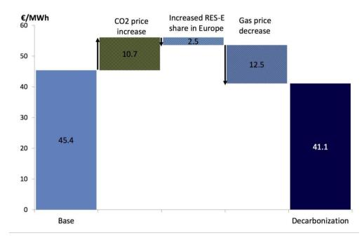
*Figure 5.5:* Step-wise development of Norway's average electricity price from the Base Scenario to the Decarbonization Scenario *Source:* Author's own illustration
