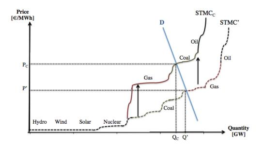
*Figure 3.7:* Fuel switch on the merit order curve *Source:* Author's own illustration
