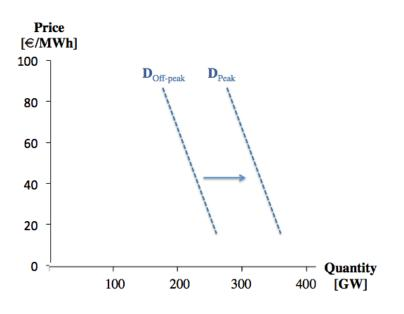
*Figure 3.2:* Demand curves for electricity in a winter-peak system *Source*: Author's own illustration.
