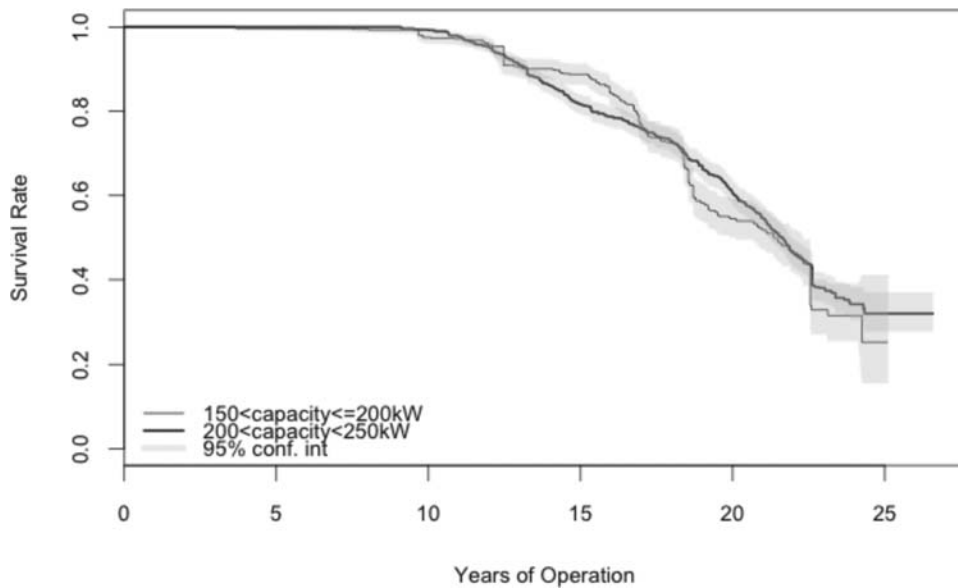
Figure 9: Survivor Function for Turbines Rated Close to 200 kW
