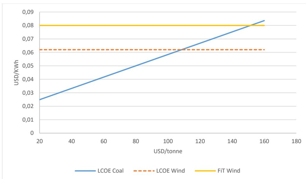
**Figure 4.10.** Coal LCOE as a function of coal price. Introduction of FiT for wind power.
