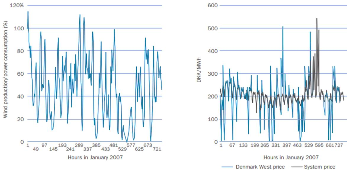
**Figure 3.4.** An example of wind resource volatility in Denmark in January 2007. Left graph shows hourly share of wind in total electricity consumption. Right graph shows spot hourly price of electricity in Danish kroner per MWh (EWEA, 2009).
