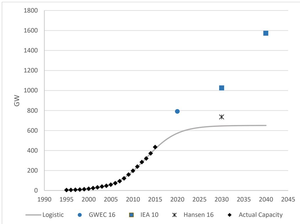
*Figure 3.3. Modelled logistic global wind capacity and its forecasts.*
