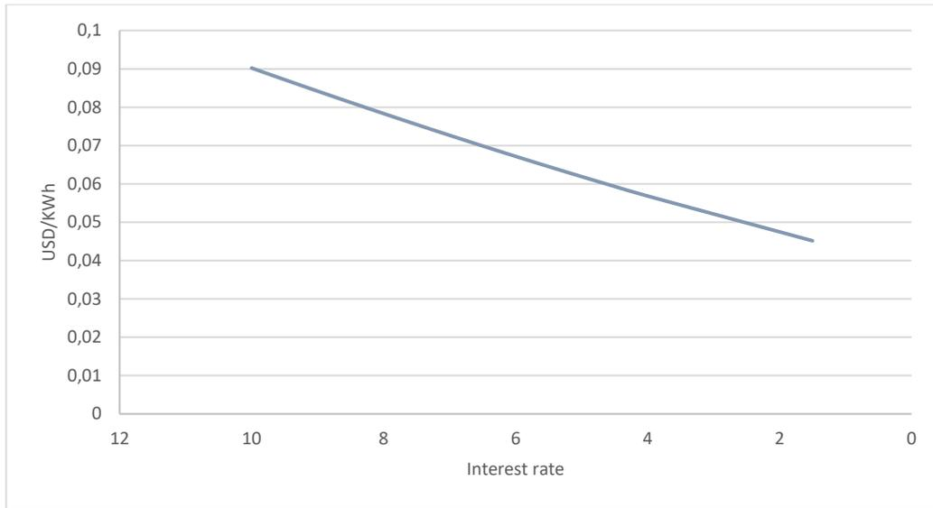
**Figure 4.5.** Dependence of LCOE on interest rate  $r$  (%)
