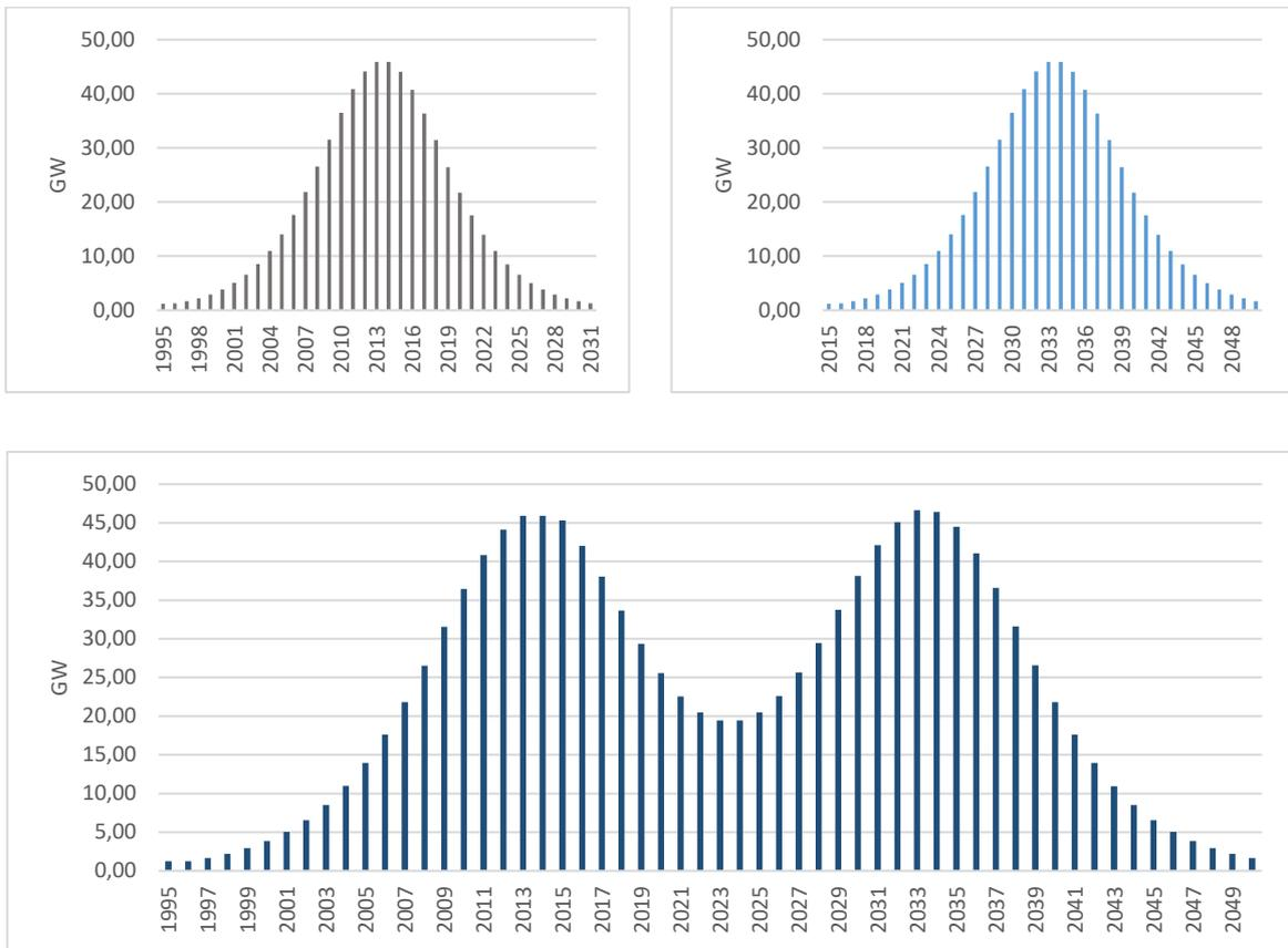
**Figure 3.5.** Modelled annual new capacity installations (grey), substitution for retired installed capacity (blue) and total annual installations (dark blue), given 20 year long life cycle.
