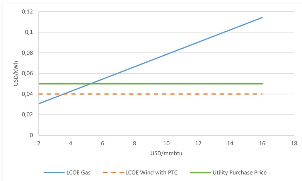
Figure 4.11. Gas LCOE as a function of gas price. Introduction of PTC for wind power.
