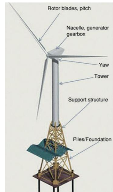
*Figure 1.1. Parts of a wind turbine (Narbel et al., 2014).*
