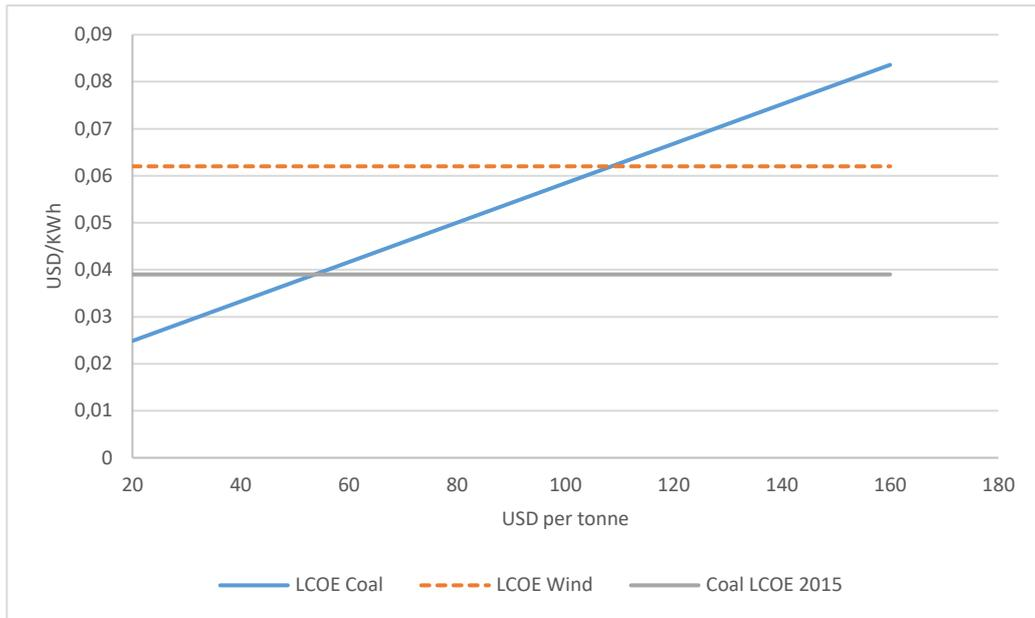
**Figure 4.7.** Change in coal LCOE as a function of coal price. Price data from BP (2016)
