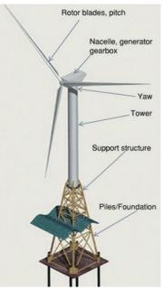
Figure 1.1. Parts of a wind turbine (Narbel et al. 2014)
