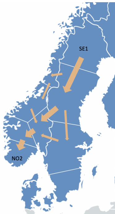
Figure 4.1: Illustration of loop flows from SE1 to NO2 (created by the authors).
