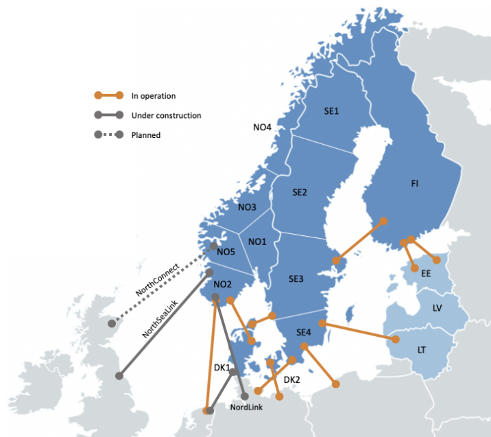
Figure 2.5: Current, future and planned cross-border HVDC interconnectors in the Nordics (European Network of Transmission System Operators, 2019).
