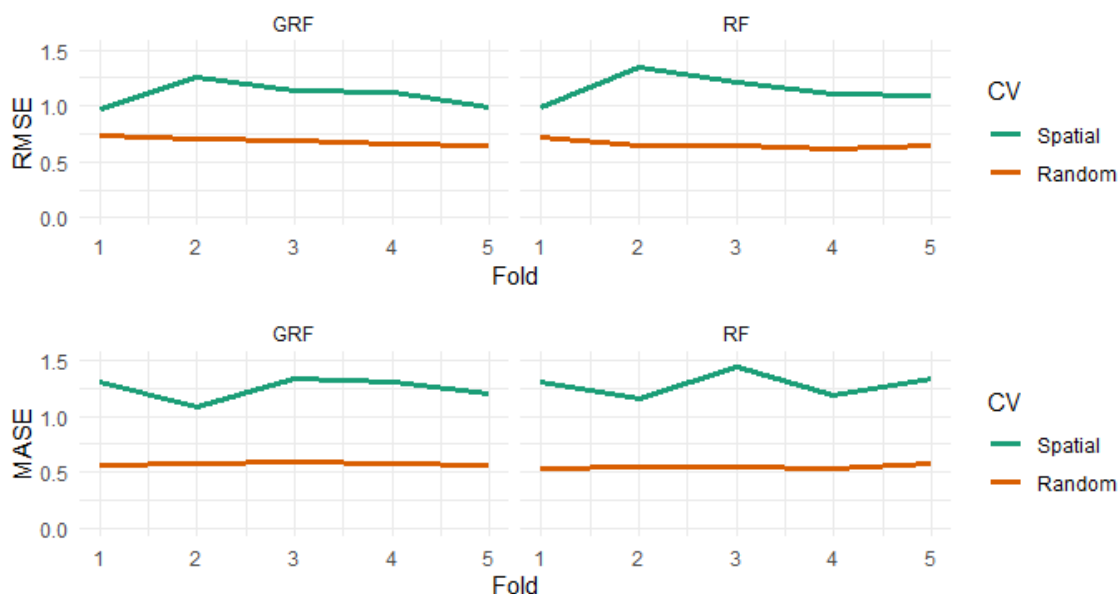
Figure 6.8. Performance metrics computed through random- and spatial CV. For spatial CV, the x-axis represents which spatially disjoint subset of data is held out as a test set. For random CV, the x-axis represents different random partitions of train/test sets.
