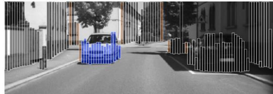
(d) Static background and moving objects are divided. The color represents a group of connected rectangles with similar motion. Brown rectangles are flagged as potentially inaccurate.
