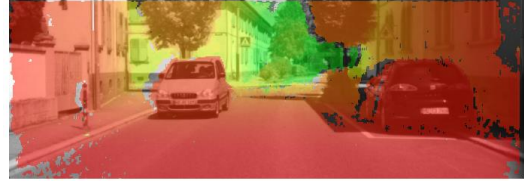
(b) Red pixels are measured as close to the vehicle (e.g. distance < 10m) and green pixels are far away (e.g. distance > 60m).
