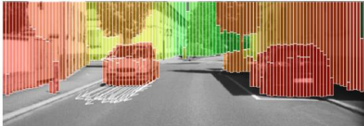
(c) Objects are efficiently described using vertical rectangles. All areas that are not covered with, are understood as potentially drivable space. The arrows in front of the approaching vehicle show the estimated object velocity. The color shows distance.
