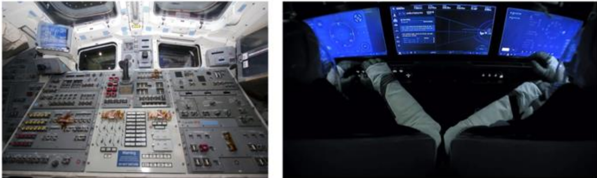
Figure 13: (Left) The traditional dashboard of the Space Shuttle Atlantis, where astronauts had more control of the spacecraft (Right) The touchscreens of the Crew Dragon capsule, designed to navigate autonomously to the ISS (Patel, 2020)
