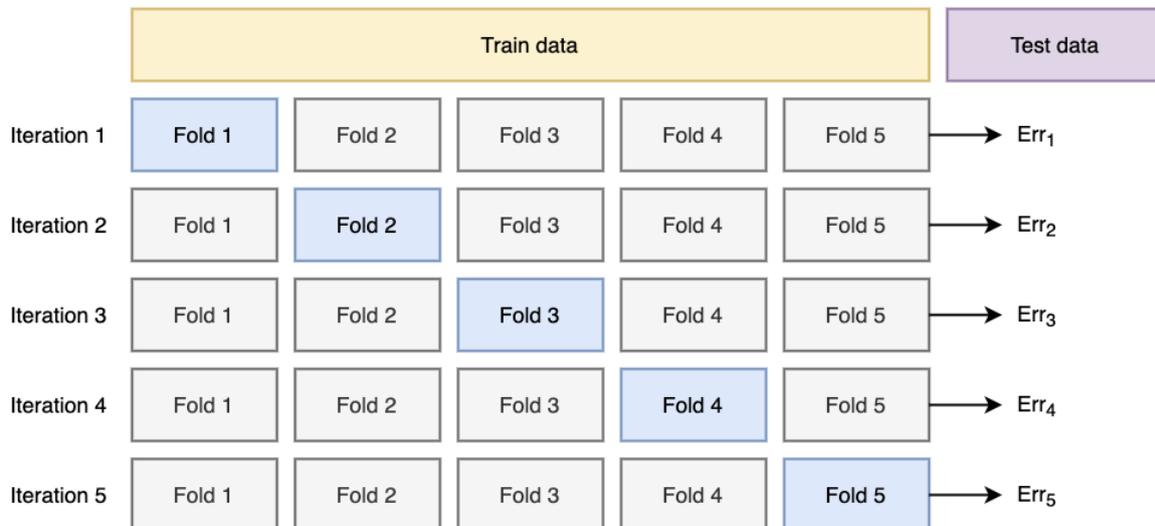
In figure 3.1 the blue folds represent the validation fold, while the four grey folds represent the folds used for estimation for each iteration. All folds are derived from the training data, seen in yellow in figure 3.1. Furthermore, the error rate for  $k$  folds when validating using the omitted folds, can be derived as follows:
