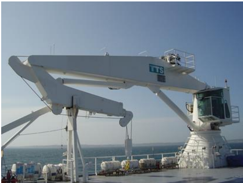
Figure 1: One of the subsea cranes that TTS offers – a knuckle boom crane (TTS, 2014d)
