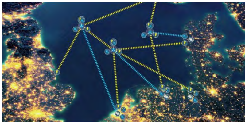
Figure 3.13 Illustration of the North Sea Wind Power Hub. Offshore wind farms are connected to artificial island or larger offshore substations ultimately connected to multiple countries through HVDC-cables (yellow lines). Production of hydrogen from surplus energy when electricity demand is low could be transported through pipes (blue lines).
