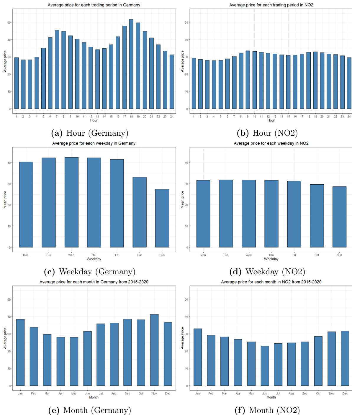
Figure 3.3: Average day-ahead prices for each trading hour, weekday, and month, in NO2 and Germany from 2015 to 2021.
