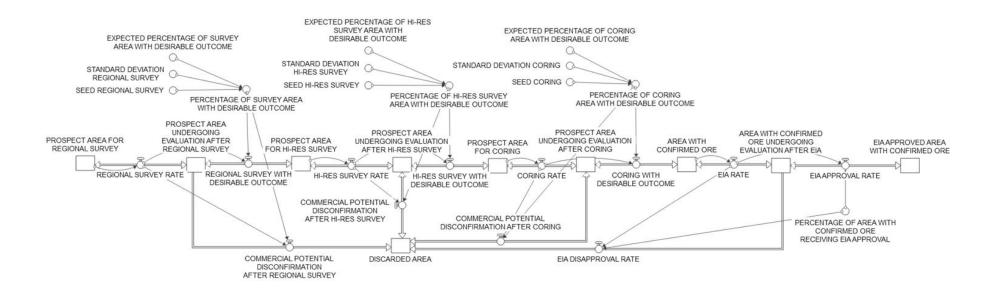
Fig. A1 Stock-and-Flow Diagram of the Exploration Process
