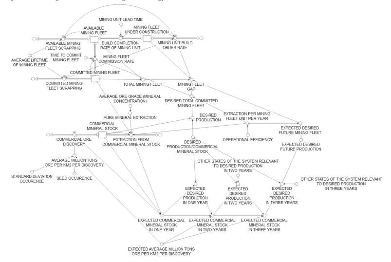
Fig. A4 Stock-and-Flow Diagram for the Mining Process and Technology
