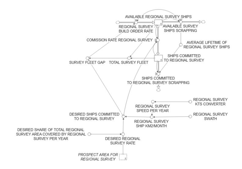
Fig. A2 Stock-and-Flow Diagram for Regional Survey Capital Structure
