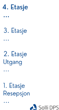
Figure A4.1: An example of a reassurance sign that is applicable for the stairway at node 1.
