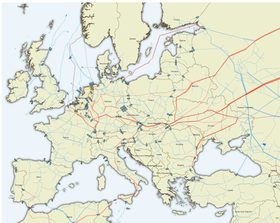
Figure 14 European natural gas pipeline network (■: transit pipeline, ■: transmission pipeline). Pipelines connecting Russia to the rest of the continent are more numerous and have larger capacity (Source: IEA.org 2014).
