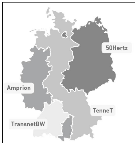
Figure 2: TSO Setup in Germany (Müsgens, Ockenfels, & Peek, 2014)
