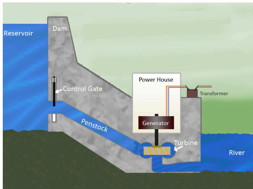
*Notes:* The figure illustrates the basics of how a hydroelectricity plant function. Water is stored in the reservoir, flows through the penstock and spins the turbine, causing electricity to be generated (Daware, 2016).
