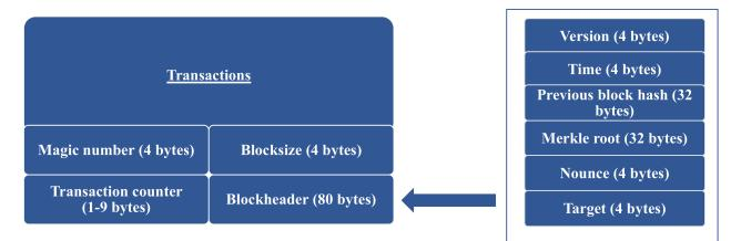
Figure 3: Block Structure (Own Illustration)
