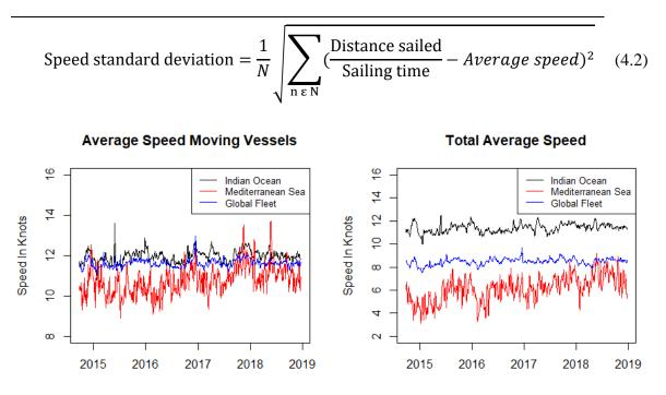
Figure 4.4 Average speed moving vessels, and total average speed.
