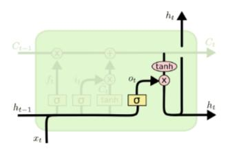
Figure A.6 Output from cell state (Olah, 2015).
