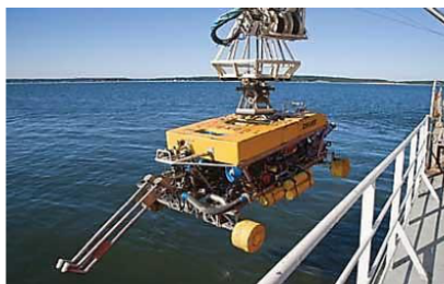
Nexans's CAPJET trenching system
