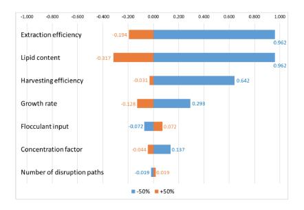
Figure 11. Sensitivity analysis results for Chlorella vulgaris, the analysis is performed by changing the parameter values one by one by  $\pm 50\%$  of the baseline value to observe the change in the total production cost (Kang et al., 2018).
