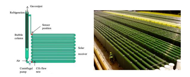
Figure 5. Photobioreactors : classical tubular system scheme (left) (Dormido et al., 2014) and representative picture (right) of commercial plant with vertical reactors in Portugal (Acién et al., 2017)
