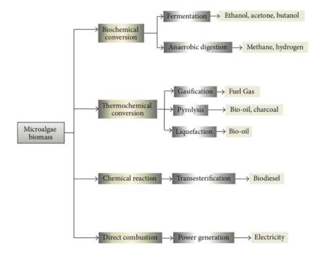
Figure 7. Microalgae biomass conversion processes (Medipally et al., 2015).
