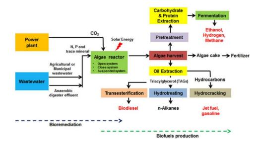
Figure 18. Example of an integrated algal culture system for the production of biofuels and coproducts (Hwang et al., 2016).
