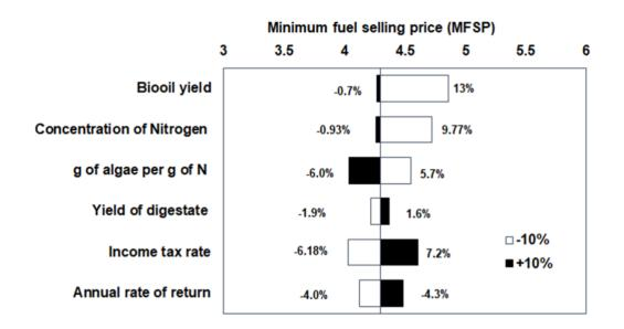
Figure 16. Sensitivity analysis on the MSP of microalgae-derived biofuel, calculated at 4.3 US \$/G (base case) (Ranganathan and Savithri, 2019).
