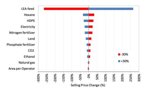
Figure 13. MFSP sensitivity analysis. Tornado plot demonstrated the extent to which algal MFSP changes with  $\pm 30\%$  of input parameters. The center line represents the baseline case. The blue and red shading bar represents the direct and reverse relationships. (Batan et al., 2016).
