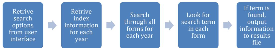
Figure 9: The simplified steps used by the program to search through SEC forms
