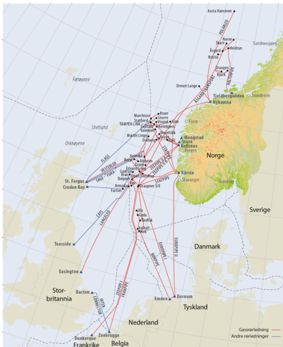
Figure 2.3: Pipeline network exporting Norwegian gas
