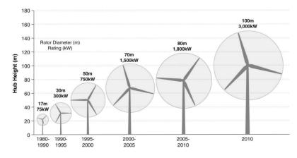
Figure 6: Development in representative turbine architecture (IEA Wind, 2012)
