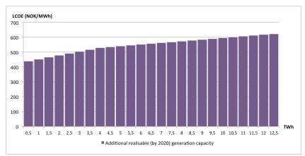
Figure 30: Cost resource curve for additional realisable (by 2020) onshore wind power projects, Norway
