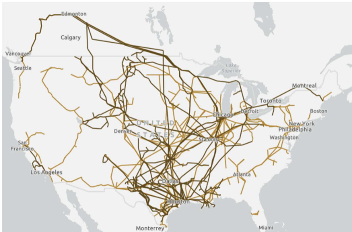
Figure 3 - Pipeline infrastructure in the US. Brown lines are crude oil pipelines, and yellow lines are petroleum products pipelines: Source: (U.S. EIA, 2023)
