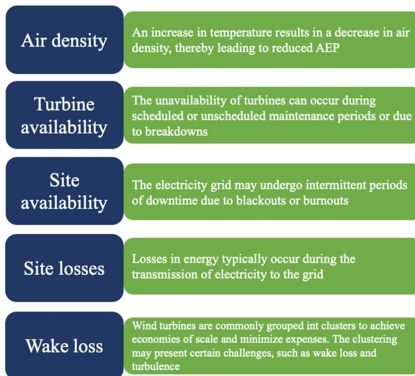
*Figure 3.12: Loss factors of an OW turbine, input from Letcher (2017)*
