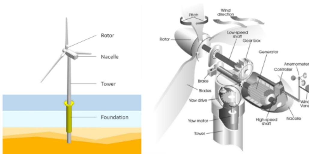
**Figure 3.14:** Components of a HAWT
