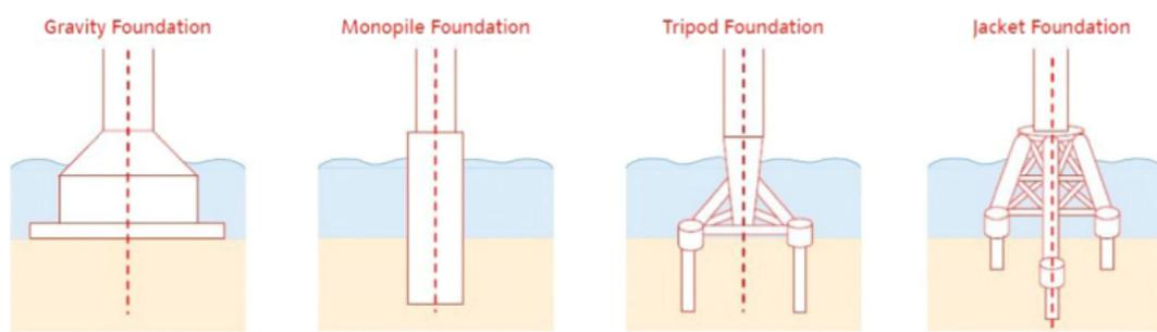
**Figure 3.16:** Some bottom-fixed OW foundations
