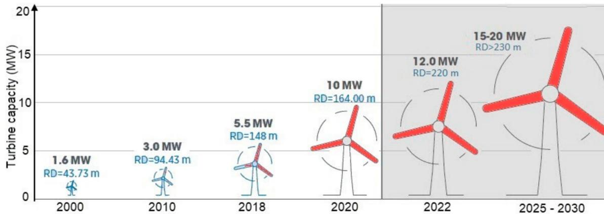
**Figure 3.15:** Development of wind turbine power and rotor diameter
