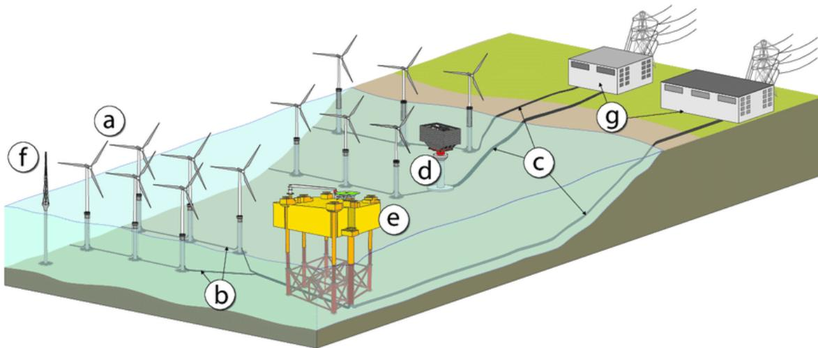
**Figure 3.13:** Main components of an OWF
