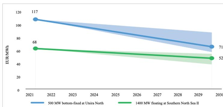
**Figure 3.10:** LCOE predictions of floating and bottom-fixed OW by NVE
