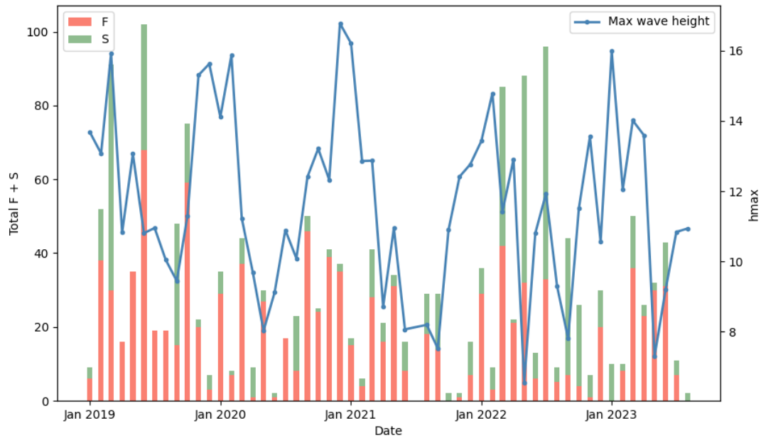
Figure 5.19: Max wave height (m) and sustained and failed components by month in the North Sea.
