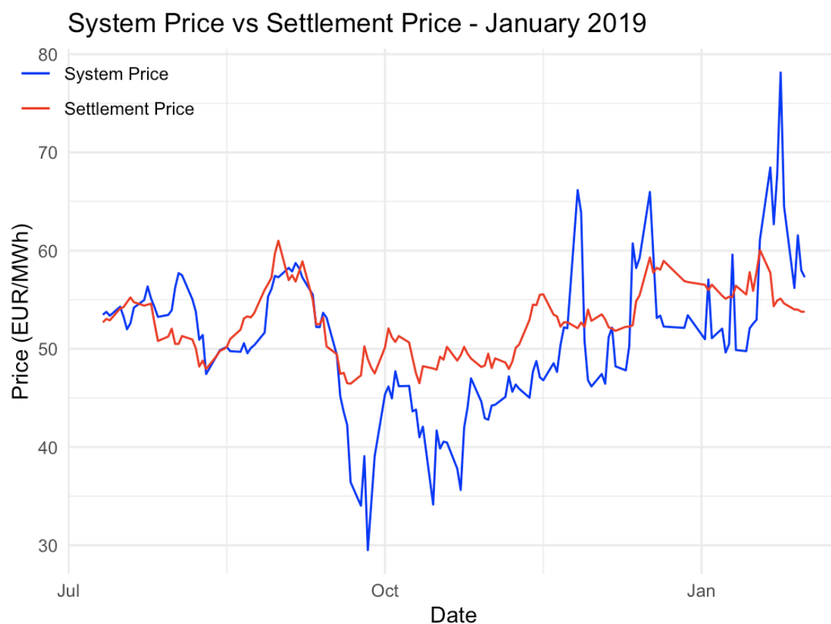
Figure 6.11: Development of system price compared to the settlement price from July 2018 - February 2019.
